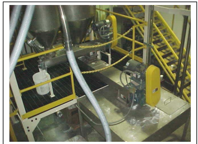
View of vacuum receivers and blending screw
